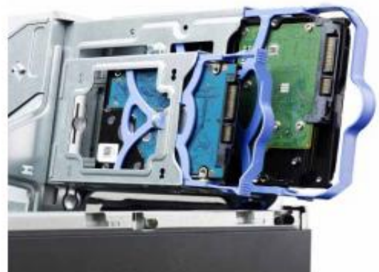
Optional 2.5" bay on Lenovo ThinkCentre M93/M93p Small Pro * Come with optional 2.5" 2nd HDD
